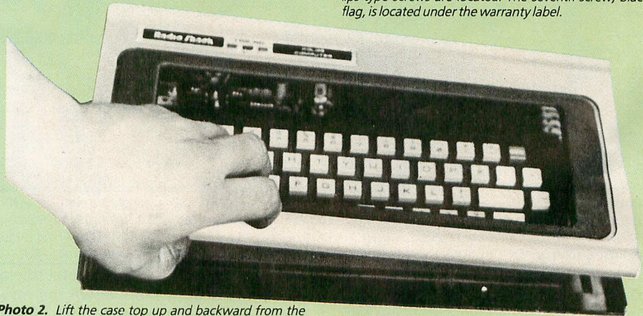
Photo 2. Lift the case top up and backward from the front; it has a plastic lip to hold it down and will snap up when enough pressure is applied.
